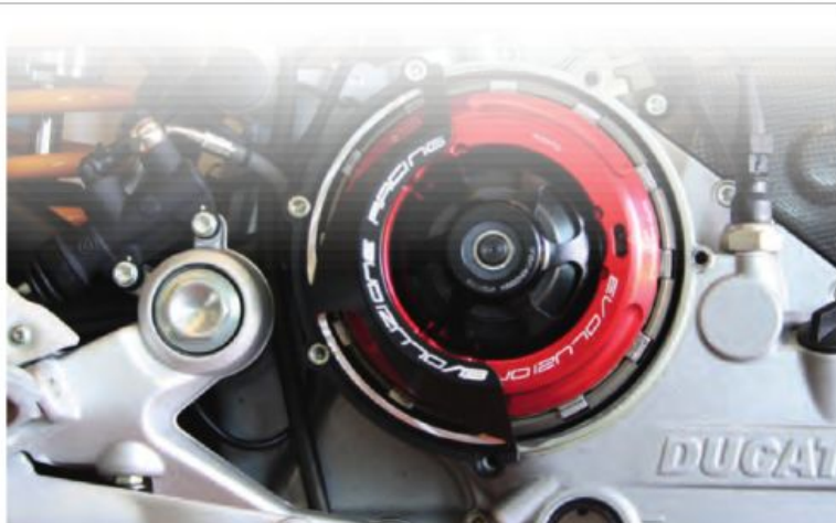
This slipper clutch system replaces the OE inner hub and pressure plate. This system keeps the OE clutch basket and OE steel plates and friction plates.
