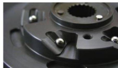
This slipper clutch system replaces the OE inner hub and pressure plate. This system keeps the OE clutch basket and OE steel plates and friction plates.
